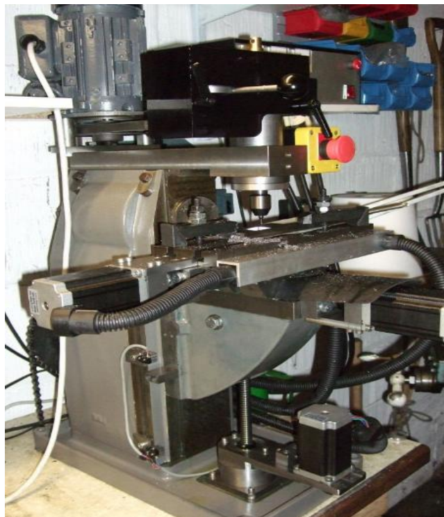
Fig. 21. Ball screw and motor mechanism to Z-axis lead screw nut holder reassembly [26]
